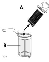
**3.** Turn the handle about 1/4 a turn anticlockwise and remove.
